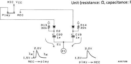
• In the mute circuit depicted above, a minute pulse is input to pin 21 as shown in the figure to switch from REC to PLAY or from PLAY to REC. At this time, current is determined by:
